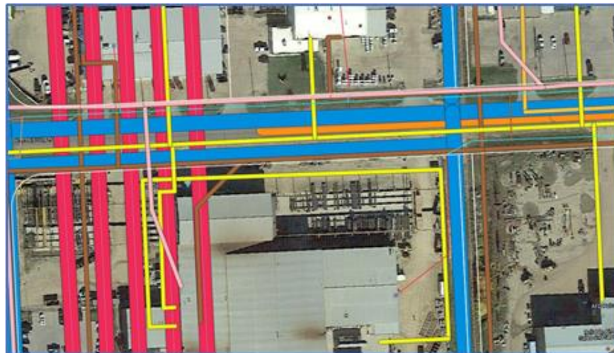
Figure 33. Including deep and shallow utility information significantly enhances design accuracy
